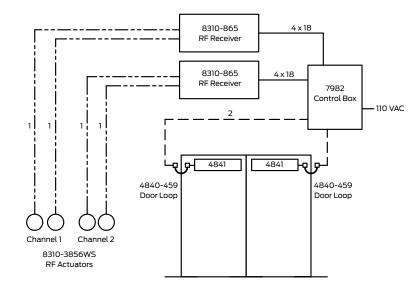
Operation: Doors normally closed, not latched. Two 8310-3856WS actuators to independently signal each door to swing.
